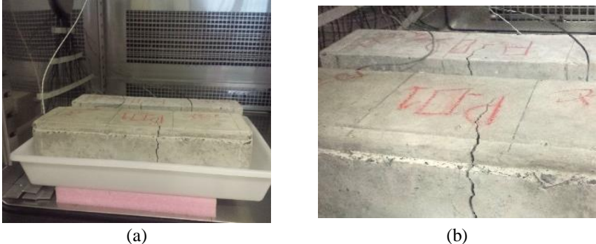
Figure 9: (a) Prismatic specimen inside the climatic chamber and damage; (b) Crack charactering the damage.
